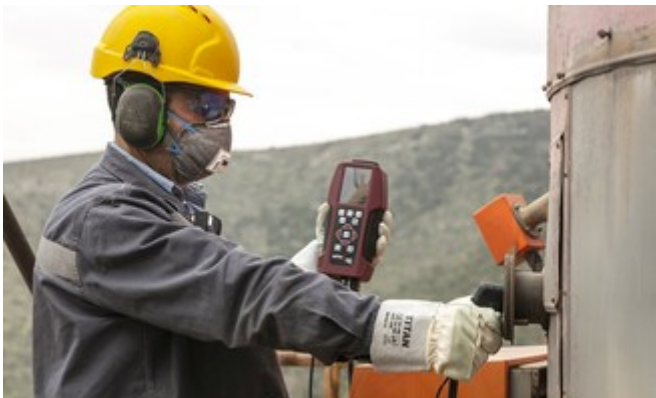
Emissions monitoring system on the chimney, Greece
